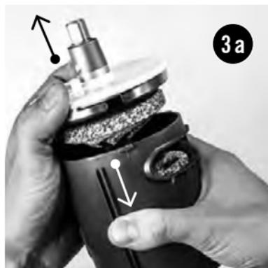
Take the flange away from the inner body in your left hand you are holding the rotor (rotating stone), in your right the stator.
