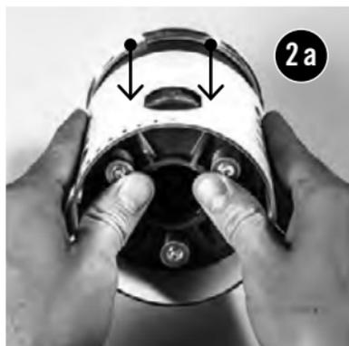
Remove the casing sleeve completely.
