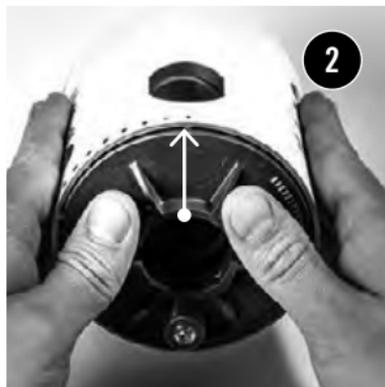
Stand the Mockmill on the three springs and pull the outer casing down around it.
