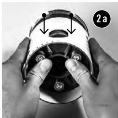
Remove the casing sleeve completely.
