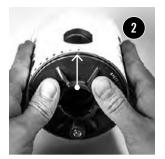
Stand the Mockmill on the three springs and pull the outer casing down around it.
