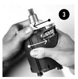
Holding the flange as shown in your left hand, turn the inner body to the right until it stops.
