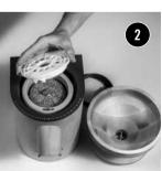
You can now lift the upper stone (stator) and control the milling surfaces
