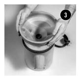
Take the hopper and turn it one full time clockwise. Then plug the mill into the power socket and switch on. Turn the mill further until you hear a slight ticking noise (first stone contact).
